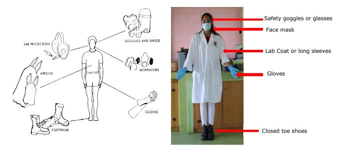
For added protection, loose clothing, neck ties, bulky rings and dangling jewellery may not be worn when working with or near moving machinery. Long hair must be tied back or enclosed in a hair net.
